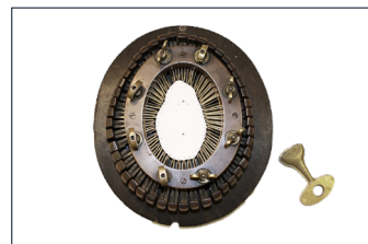
The Formillion is placed over the pattern. The pins are adjusted to match and then tightened.
