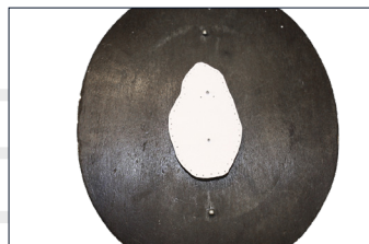
The pattern is fixed onto the wooden base.
