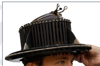
Its arms adjust to the head; pins above create a perforated paper pattern. This reduced pattern is cut out and then enlarged to the correct scale using a Formillion.
