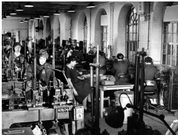
Umbrella Department, Samuel Fox and Co. Ltd., Stocksbridge Works showing women operating the multi-stage machines used in the making of umbrella ribs and stretches (1940-1959).
