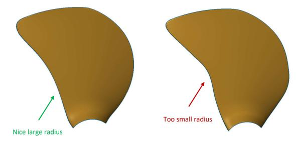
The blade geometry is defined by several parameters. The shape of the trailing edge is represented by the curve LA, that has a linear relationship LA = 0.5\*L+SKEWL to parameters (curves) L and SKEWL.
