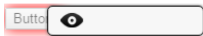
Figure 29. The eye icon is used to make hidden objects visible on the TP screen
