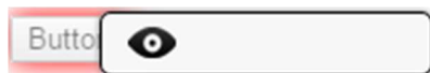
Figure 29. The eye icon is used to make hidden objects visible on the TP screen
