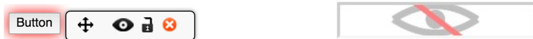
Figure 20. (a) Clicking the eye icon hides objects. (b) Hidden input fields get a special symbol
