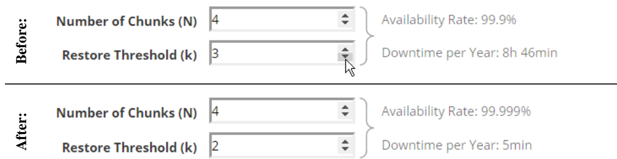
Figure 14. Immediate feedback when the user changes the value on the default values on N and k .
