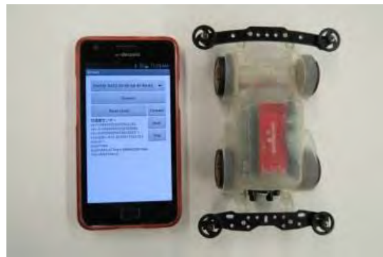
Figure 1 Device driven by application using acceleration sensor and shuffling movement
