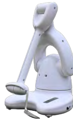
Figure 1. The eating aid device Bestic [9].
