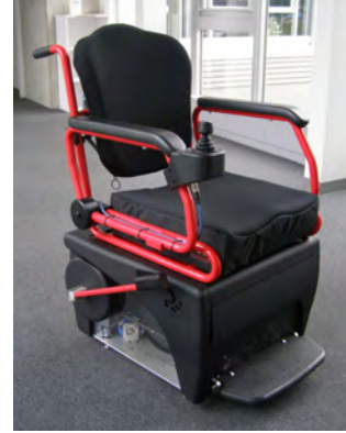
Fig. 2. Prototype of a dynamically stable wheelchair of single spherical drive (Spheel)
