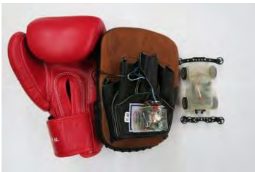
Figure 7 Device driven by hit a mitt
