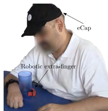
Fig. 1. The robotic extra-finger is used to compensate hand grasping abilities for patients suffering from sensorimotor hand impairment).
