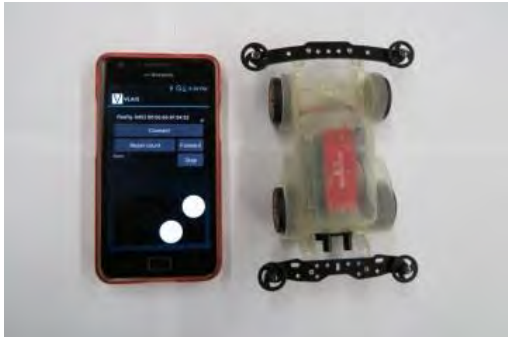
Figure 6 Device driven by tap the screen of the smartphone
